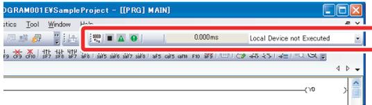
The ON/OFF status of bit devices can be checked on the ladder screen.
